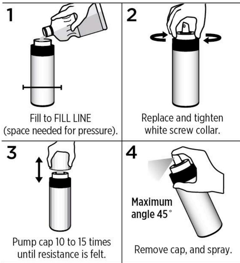
At full pressure, MISTO will spray for about 15 seconds before needing to be pumped again.
